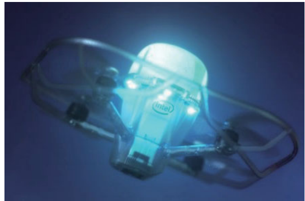
Figure 2 Intel Premium Drone, a Purpose-built Drone for Light Shows (©2021–Intel Corporation)
