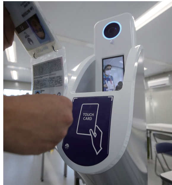
Figure 1 Olympic ID Card Presented to Advanced Access Control System (©2021-International Olympic Committee-All Rights Reserved)
