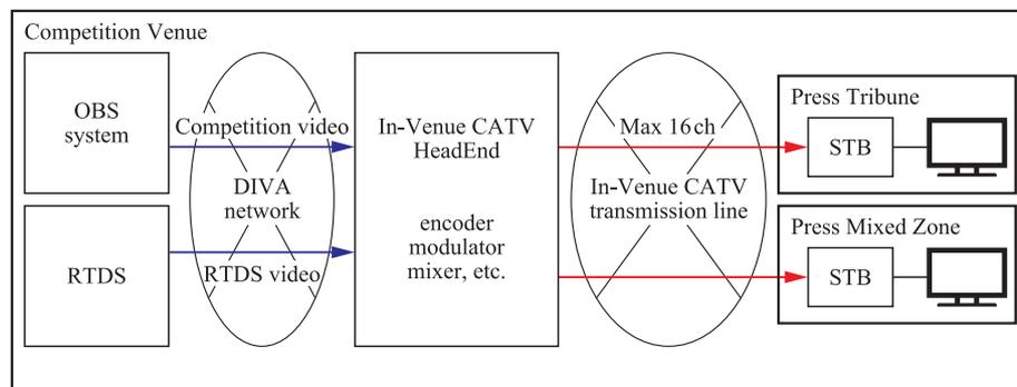
Figure 4 In-Venue CATV System Configuration The figure shows the system in the form of RF signal transmission. In addition, HD-SDI signals from the OBS system and Real Time Data System (RTDS) are transmitted as they are. The competition video and RTDS video were received via DIVA network, a video and audio network within the competition venues, and distributed to the TVs within the venues.
