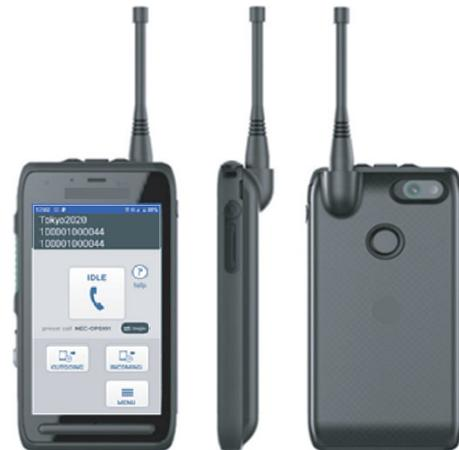
Figure 4 Mobile station A Smartphone-type Radio was Used.
