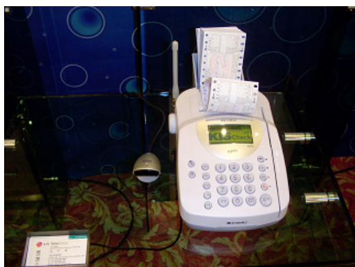
Fig.4 IrDA dongle attached to the existing POS
