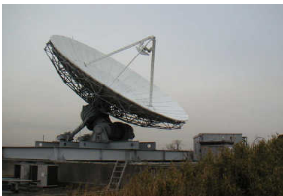
Figure 2: Experimental earth station antenna for 20/30GHz bands with 11.5m diameter.
