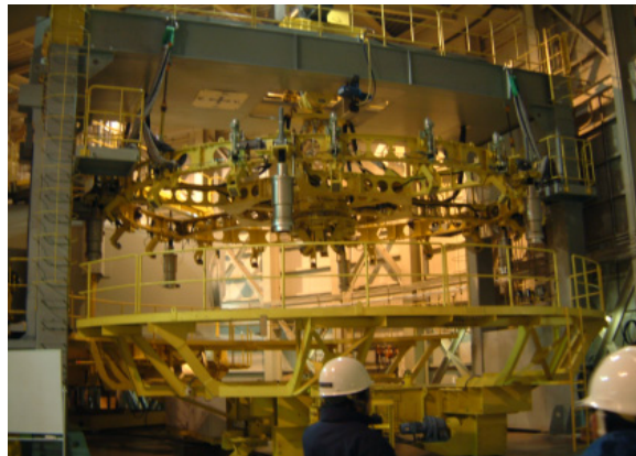
Fig. 8 Attachment for movement of primary mirror.
