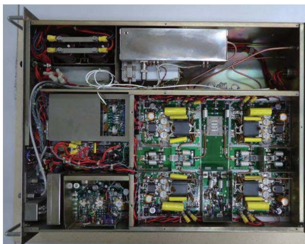
Fig. 3 Transmitter-receiver module of the MU radar
