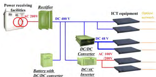
Fig. 2 Usage example of PCE in NTT's ICT facilities
