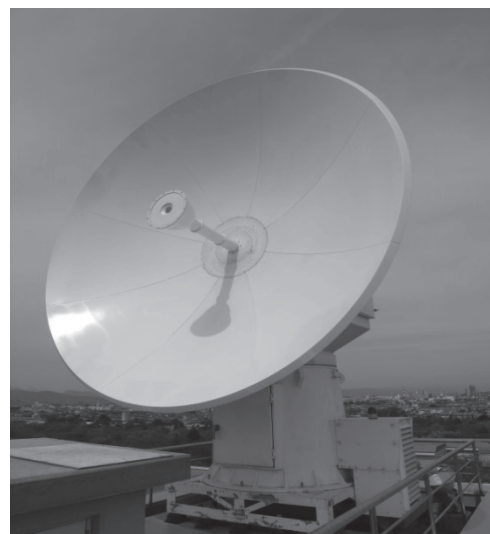
Fig. 8 S/X dual band 3.8 m antenna at Sagamihara campus of ISAS/JAXA
