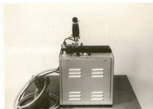
Fig. 5 Fusion splicing machine used for FR1 (This machine is about 20kg in weight)
