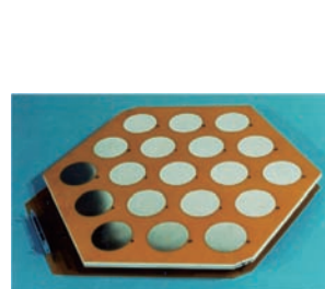
Fig. 7 First type of L-band land mobile PAA
