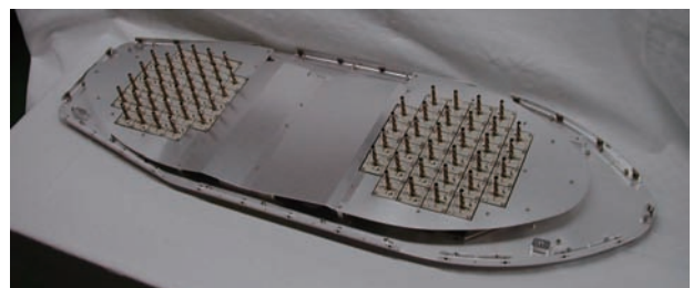
Fig. 10 S-band aeronautical satellite communication PAA
