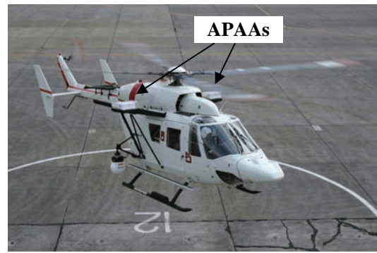
Fig. 12 Ku-band experiment helicopter-satellite communication system
