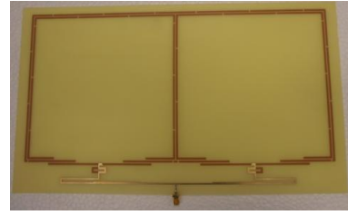
Fig. 4. Photo of the antenna prototype using the FR4 substrate.
