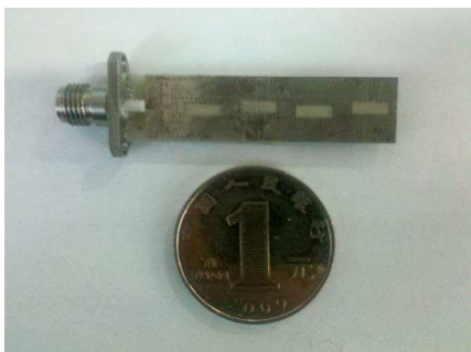
Fig 6. Photograph of the antenna array.
