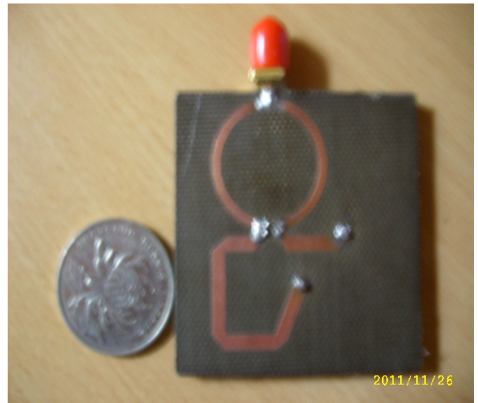
Fig 2(b)The feeding network
