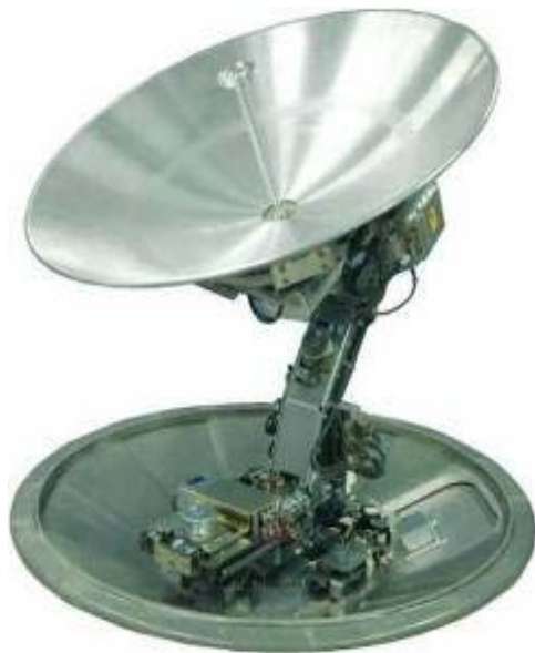
Figure 2. 120cm antenna (high gain type).
