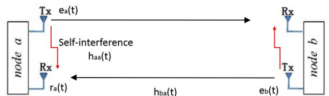
Figure 1. A simple model of full-duplex system
