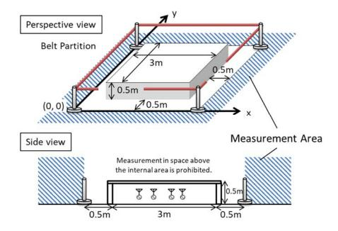
Figure 1 Setup of the transmitters and measurement area.
