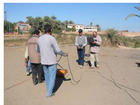
Figure 1. GPR system using metallic cables.
