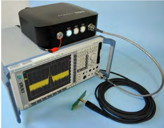
Figure 2. Helical antenna operating at 915 MHz connected to an isolating RF-over-fiber transducer and with a spectrum analyzer to remotely receive the signal.
