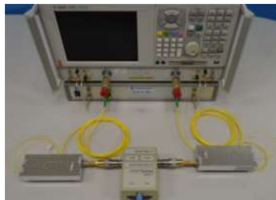
Figure 2. Photo of Our newly proposed optical fiber link port extender with VNA
