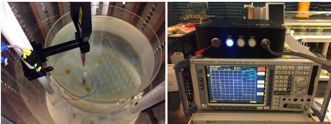
Figure 3. Left: RFoF1P4MED measurement setup inside the MITS1.5 (ZMT ZurichMedTech AG, Switzerland) MRI birdcage. Right: Measured radio-frequency signal at the output of the Remote Unit (SPEAG, Switzerland) opto-electrical converter.
