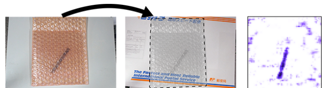
Fig. 5 Optical images of (left) Target of a cutter blade for detection in a cushioning envelop and (middle) the cushioning envelop in an EMS envelop. (right) Obtained W-band transmission image through the EMS envelop is shown. The location of the contained cushioning envelop is indicated with translucent image and dashed lines.
