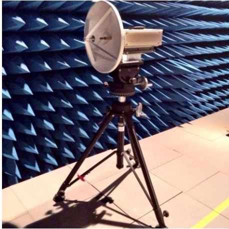
Figure 5 External view of W-band radio access unit.
