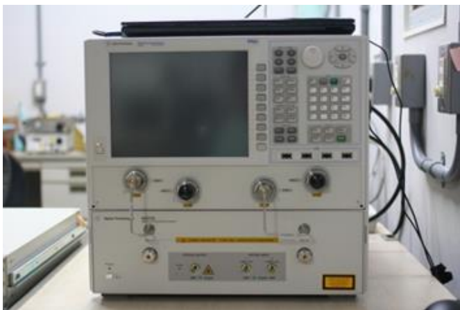
Fig. 3 N4375D Optical component analyzer of Keysight technology Inc.
