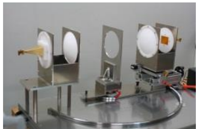
Fig. 5 Set up of free-space method
