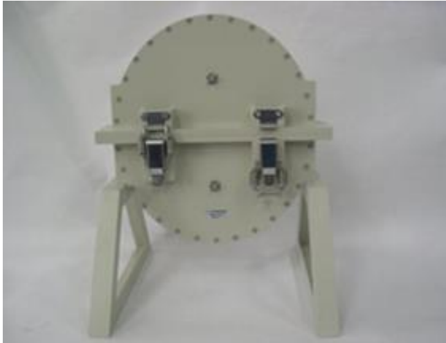
Fig. 6 Dual-Focus Flat Cavity(DFFC) for electromagnetic shielding effect measurement in the frequency range from 1 GHz to 15 GHz
