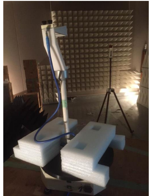
Fig. 4 Azimuth table for antenna measurement
