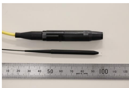
Fig. 1 Sensor tips of LeoProbe. Light source and signal processing unit is not shown.
