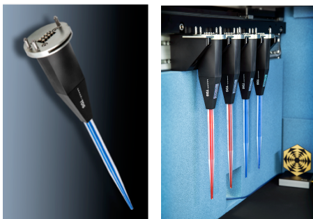
Fig. 2 TDS probes for the measurement of electric (blue) and magnetic (red) RF fields optimized for near-field scanning usage. Shown on the left are the probes located in the probe repository inside the developed near-field scanning system. A single E-field probe with a detailed view of the fiber optic machine adapter that allows up to 25,000 probe matings is shown on the right.
