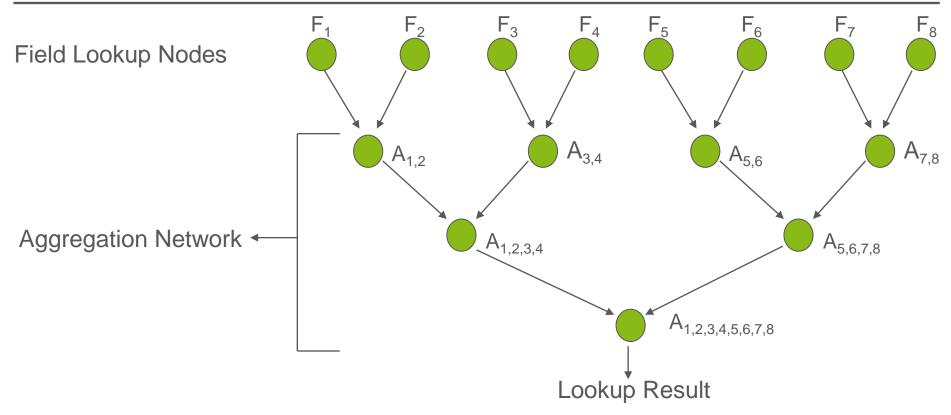
Packet header is decomposed into individual fields and fed to the classifier
