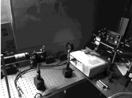
The experimental setup included a He-Ne laser with an average output power of 30 mW at 632.8 nm. A collimator and a lens of f = 200 mm was used. A L3B00Z-G84G liquid crystal spatial light modulator of Epson make was utilized for focusing the laser beam onto the ORGA VLSI. The reconfiguration time was measured by implementing a measurement circuitry on the VLSI chip and the result is shown below:
