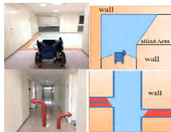
Fig 1. Example of blind area
