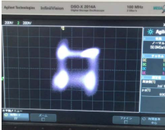
Figure 5: Phase planes between the output1 and output2 with the gaussian noise input. The Lissajous curve are closed.
