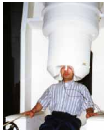
Fig.1 Steady-state multisensory evoked neuromagnetic fields were measured simultaneously by a whole-cortex MEG system.
