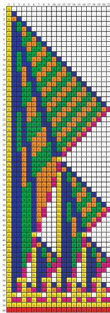
Figure 7: Configurations of a 12-state 236-rule implementation of one-sided recursive (3n - 3) -step synchronization algorithm on 21 cells.
