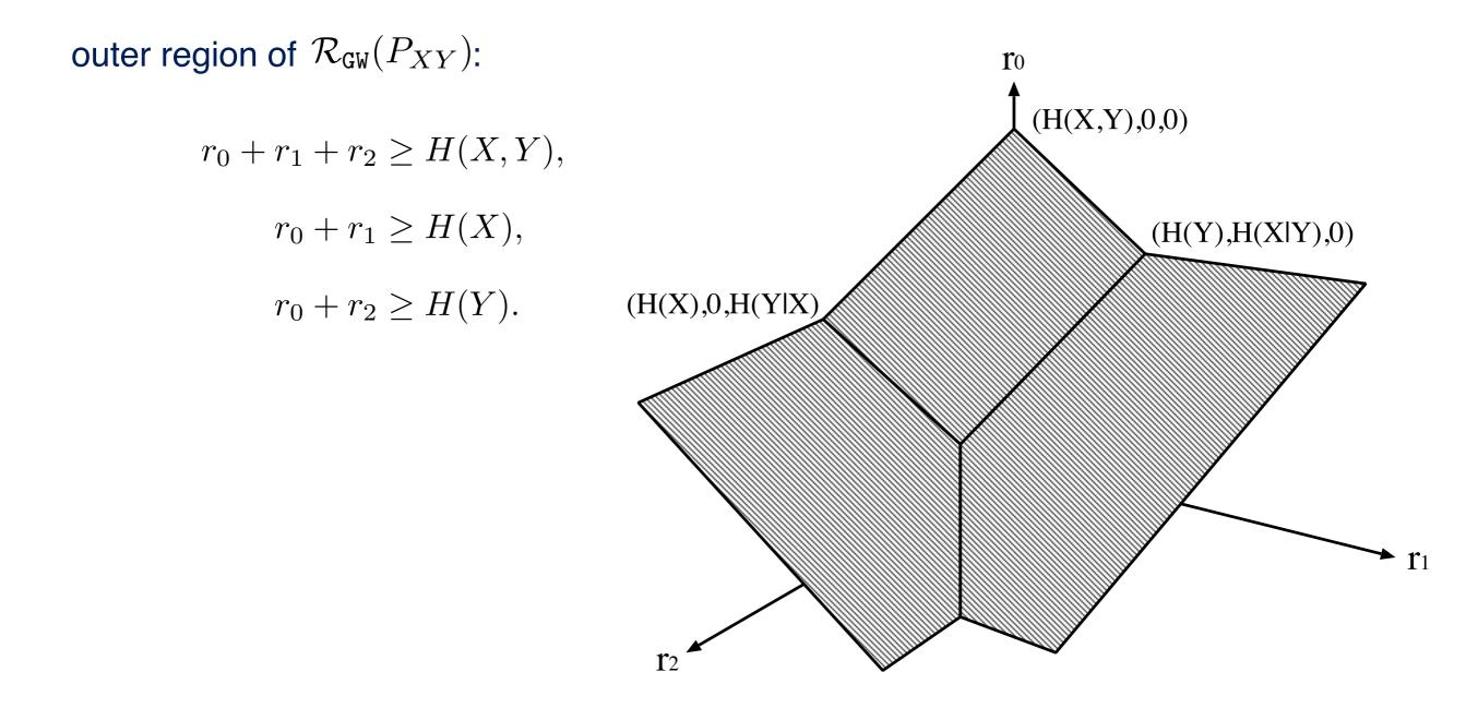
$\begin{aligned} \mathcal{R}^*_{\mathsf{GW}}(P_{XY}) &: \text{the set of all rate triplets s.t.} \\ \exists P_{W|XY}, \quad |\mathcal{W}| \leq |\mathcal{X}| |\mathcal{Y}| + 2 \\ r_0 \geq I(W \wedge X, Y), \\ r_1 \geq H(X|W), \\ r_2 \geq H(Y|W). \end{aligned}$
