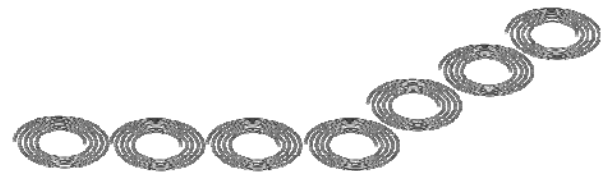
(a) Array of resonator in a bended line.
