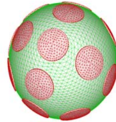
Figure 4. A conformal array of circular patch antennas mounted on the surface of a dielectric sphere with a perfectly conducting core. Both the number of elements and the radius of curvature of the surface can be large.
